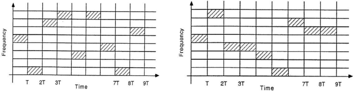
Figure 2.2 Markov (left) and Memoryless (right) based hopping patterns
