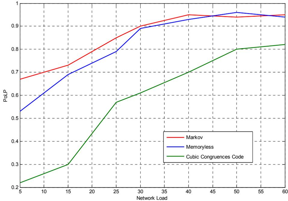
**Figure 4.5 System  $PoLP$  vs the network load for three different FH code sets ( $N=3$  and no external to system interference was considered)**
