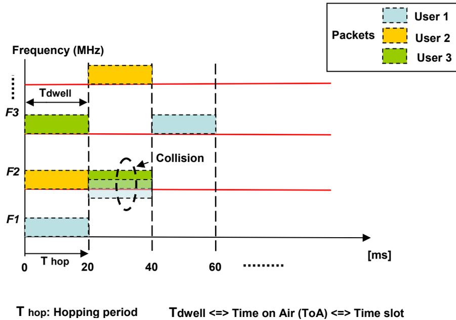
Figure 3.3 Synchronous FHSS-MA scenario with ideal clocks
