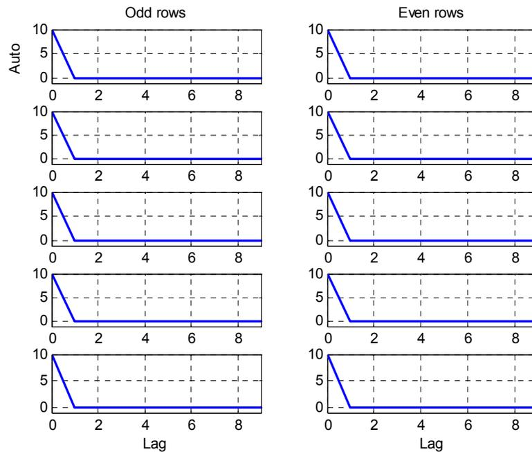
**Figure A.3 Hamming autocorrelation functions for each sequence in the CC code matrix shown in Figure A.1**
