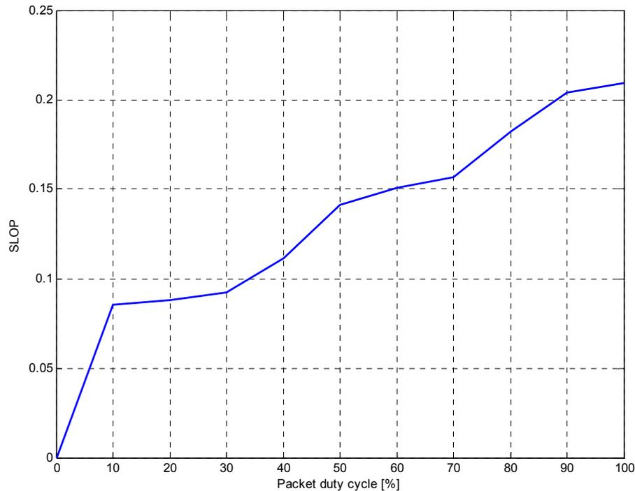
**Figure 4.4  $SLOP$  vs packet duty cycle (15 users, 40 RF channels, and  $\alpha=50\%$ )**
