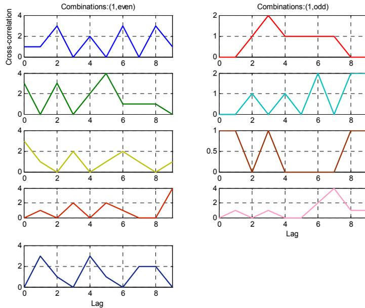
**Figure A.8 Hamming cross-correlation functions for the combinations of row one with the rest from the set of Markov codes shown in Figure A.2**
