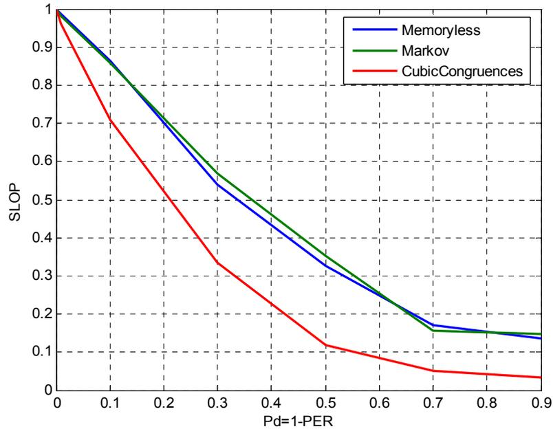
**Figure 4.7  $SLOP$  vs  $P_d$  for Markov, Memoryless and CC FH code sets (40 RF channels, 15 users and interference is considered)**
