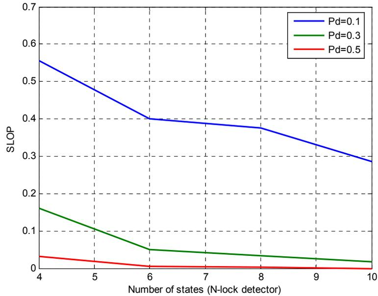
**Figure 4.2**  $SLOP$  vs  $N$  for SFHSS-MA with ideal clock scenario (15 users and 40 RF channels)
