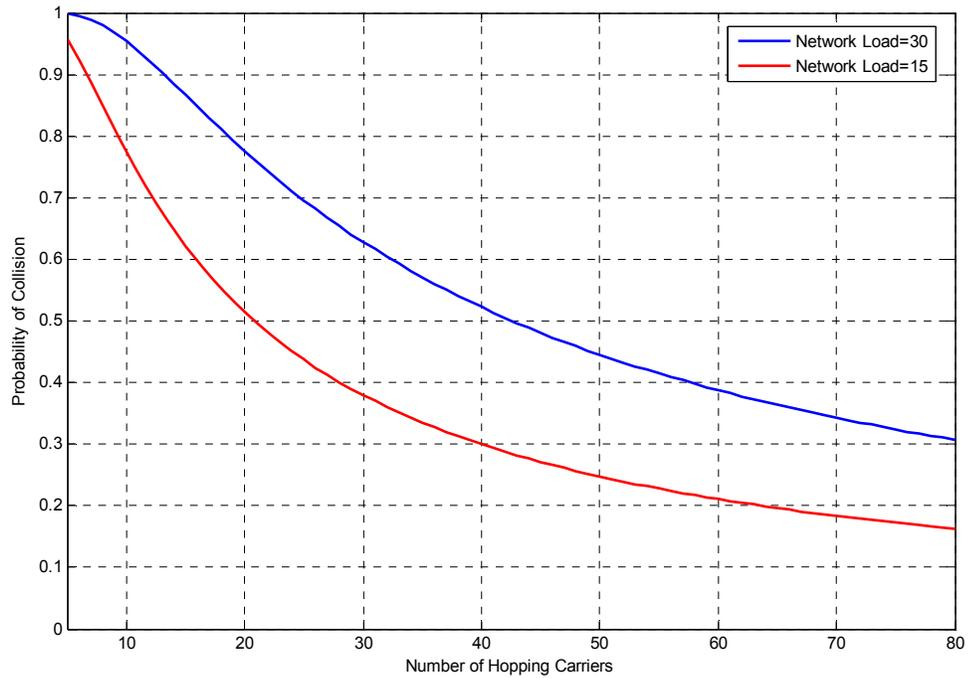
**Figure 3.4 Dependency of probability of one user being hit by the rest of the active users in the network as the number of RF channels is changed (theoretical)**
