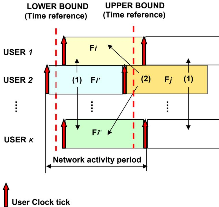
Figure 3.9 Kernel of collision analysis for SFHSS-MA with real clock case
