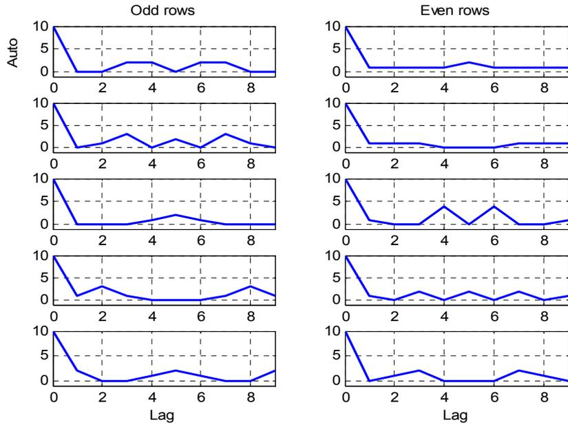
Figure A.5 Hamming autocorrelation functions for each sequence in the Memoryless code matrix shown in Figure A.2
