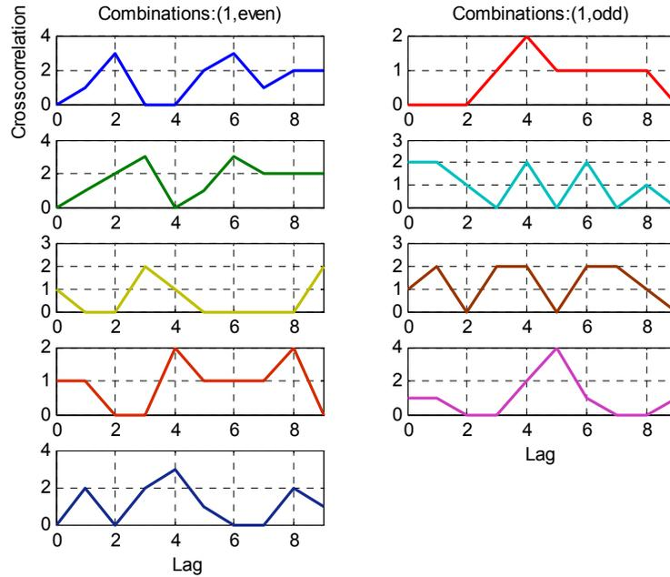
**Figure A.7 Hamming cross-correlation functions for the combinations of row one with the rest from the set of Memoryless codes shown in Figure A.2**
