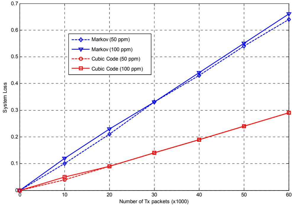
**Figure 4.6 System *PoLP* vs elapsed time for two kinds of FH code sets and clock accuracy (40 RF channels, 15 users, N=3 and only MAI was considered)**
