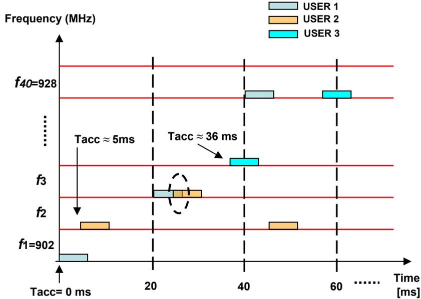
Figure 3.14 Asynchronous FHSS-MA scenario. Packet duty cycle: 30%
