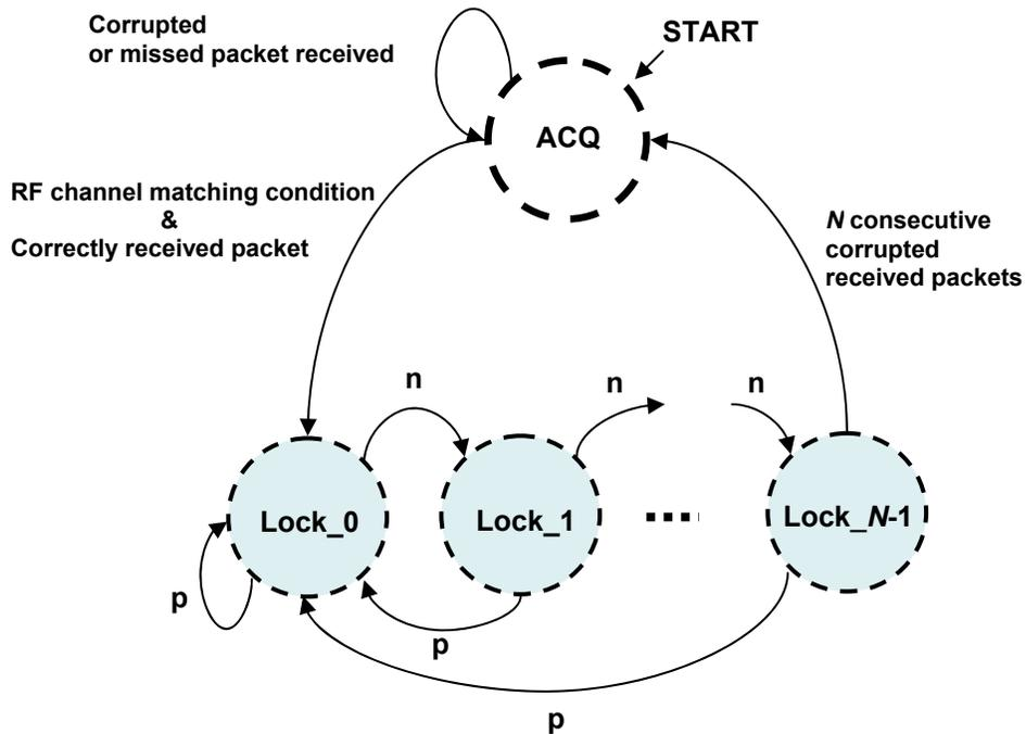
**Figure 2.5** FSM diagram associated with the modified transmitted reference synchronization algorithm for the receiver system
