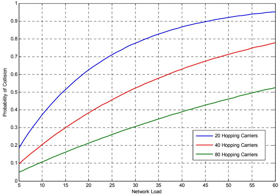
**Figure 3.5 Dependency of probability of one user being hit by the rest of the active users in the network as the network load is varied (theoretical)**
