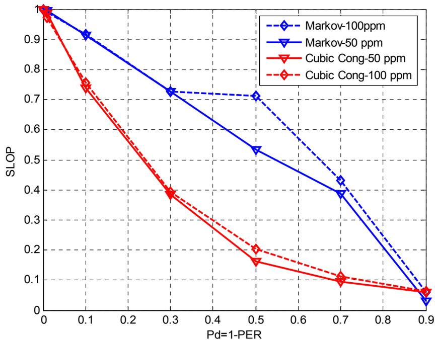
**Figure 4.9 *SLOP* vs Pd. Dependency as the clock initial accuracy is varied (40 RF channels, 30 users, and interference is considered)**
