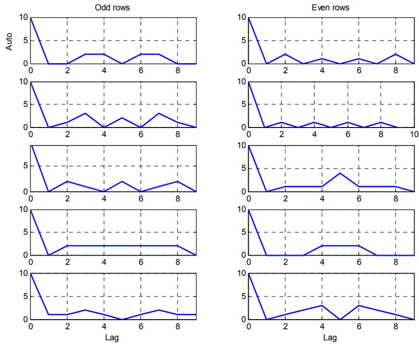
Figure A.6 Hamming autocorrelation functions for each sequence in the Markov code matrix shown in Figure A.2
