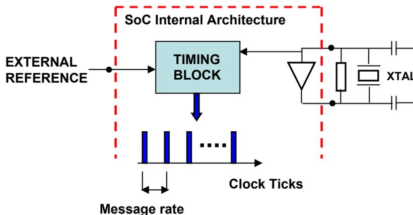
Figure 3.6 Typical timing system seen in most ISM low-power SoC
