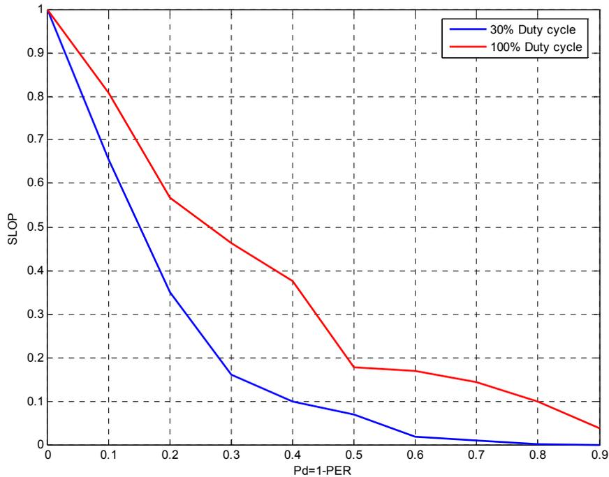
**Figure 4.3 *SLOP* vs *Pd* for AFHSS-MA with ideal clocks (15 users and 40 RF channels)**
