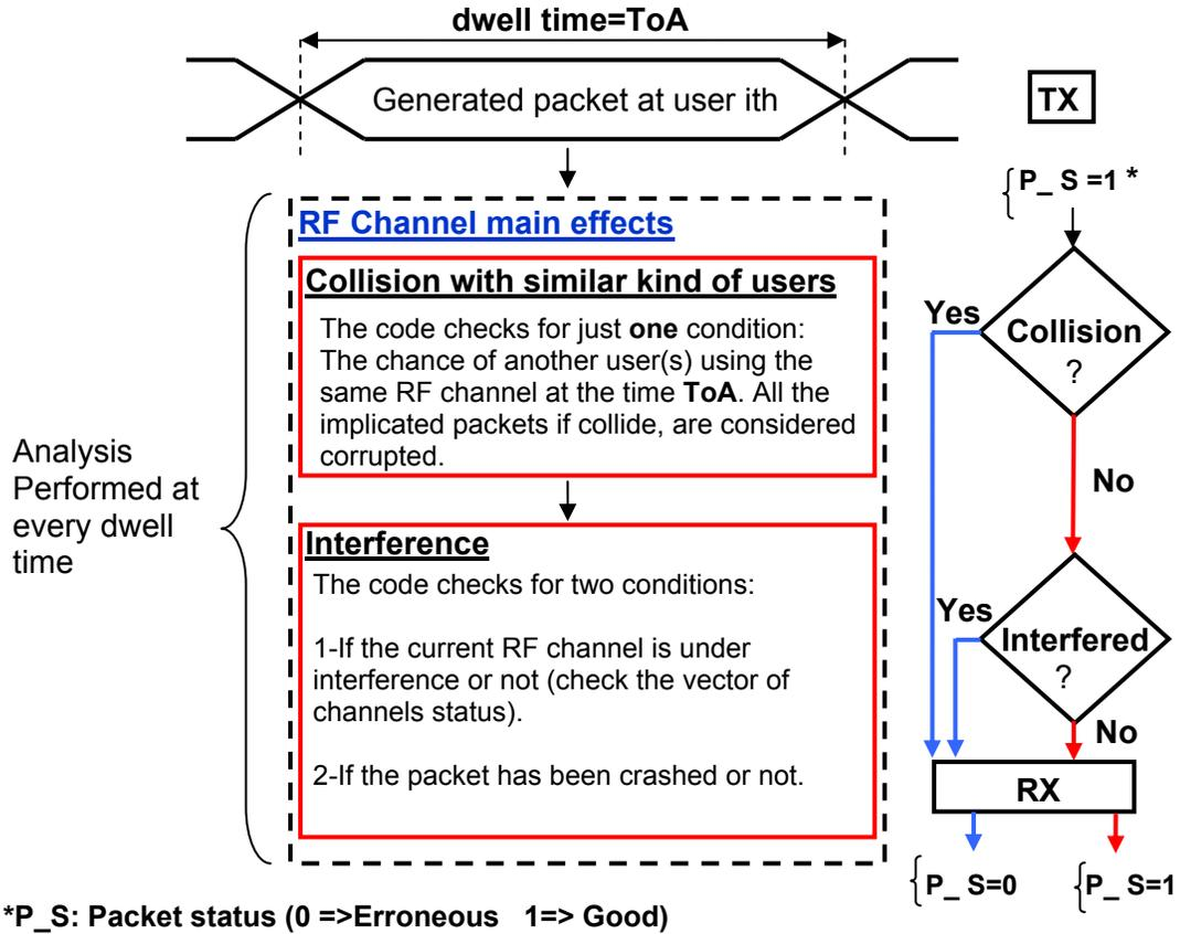
Figure 3.2 Analysis performed on a packet as it is generated at the transmitter (TX) and reaches the receiver (RX). The blue and red paths are complementary to one another’s implications
