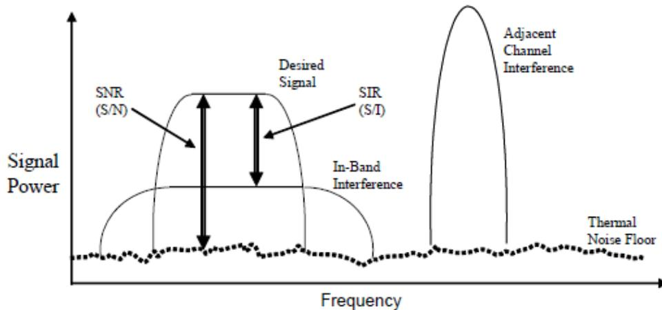
Figure 3.10 Interference scenario for a typical wireless ISM application [34]
