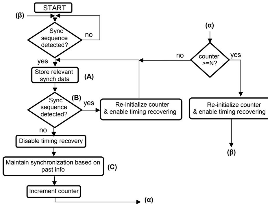
Figure 2.4 Modified transmitted reference synchronization algorithm [17]
