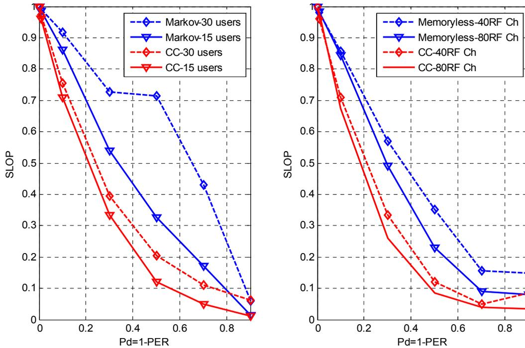
**Figure 4.8** *SLOP* vs Pd. Dependency as the network load is varied (left). Dependency as the number of channels hopping is varied (right)
