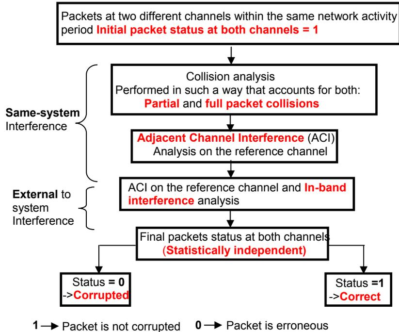
**Figure 3.12 Algorithm for the collision and interference analysis in the slow SFHSS-MA scenario with real clocks**
