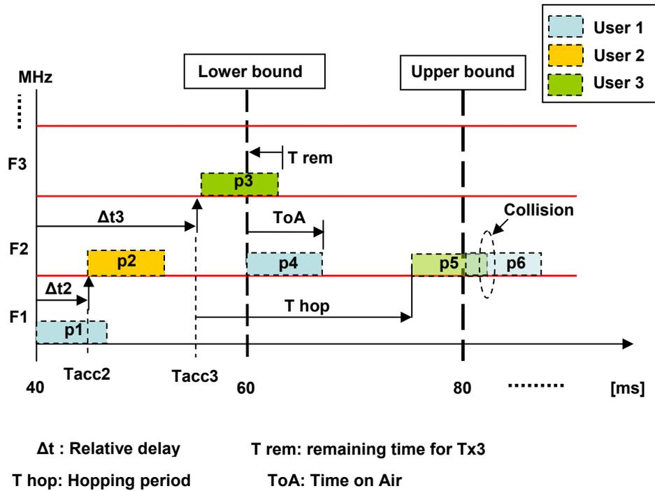
Figure 3.15 Timing diagram supporting the asynchronous model
