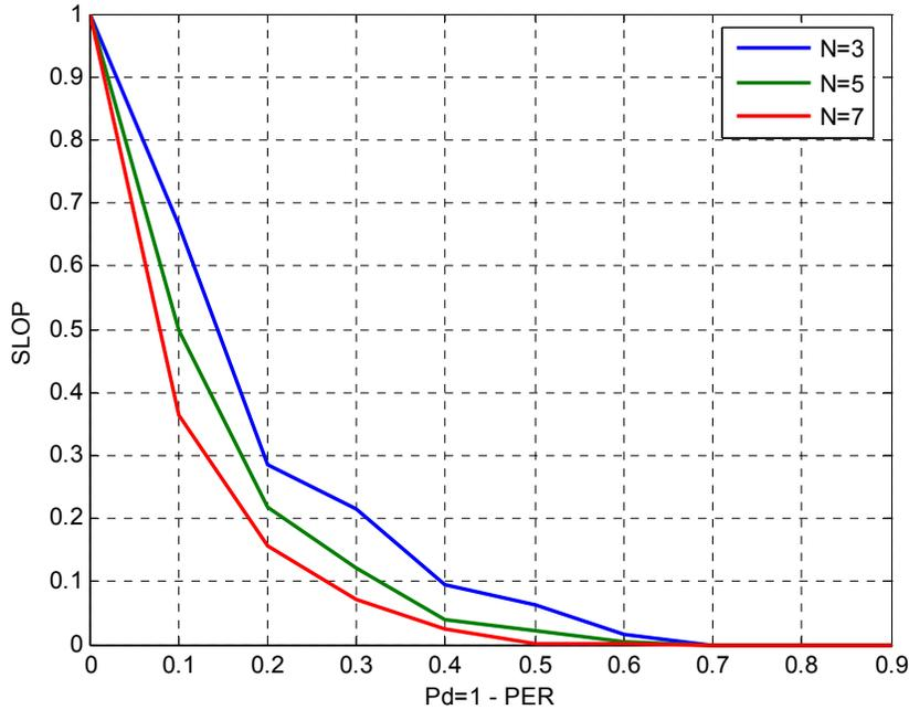
**Figure 4.1** *SLOP* vs *Pd* for SFHSS-MA with ideal clock scenario (15 users and 40 RF channels)
