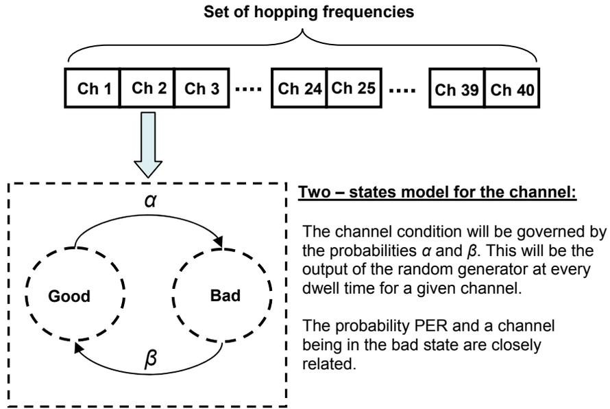
**Figure 3.1 Model for the channel as interference is considered**
