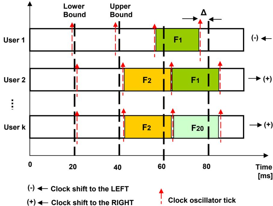
Figure 3.7 SFHSS with imperfect clock. Values ( $F$ ) represent current RF channels that are used to transmit the packet
